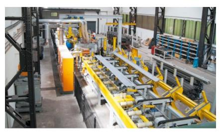
A combination of inductive material heating, continuous coating and a special drawing process reduces just the steel consumption by 124 tons a year.
