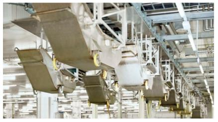
Raw products are transported to the respective production facility in transport containers via conveyor belts. Allergenic residues emerge during purification.
