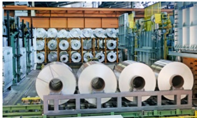
Charging machines can bring four coils at any time into the new furnace.
